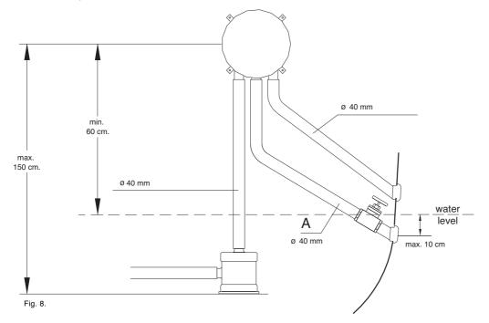
If the through-hull exhaust outlet has to be mounted far (total length exhaust piping from generator to top of goose neck (waterseparator) is more than 3 m) from the generating set, an exhaust/water separator must definitely be installed. The sea water from the
