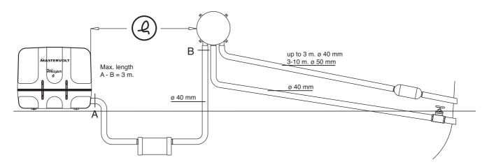
If the generating set and the exhaust system have been installed correctly, neighboring boats will not be disturbed by generating set noise, With the "super silent" exhaust system, generating set noises are almost inaudible. For optimal noise reduction, the sea water outlet from the exhaust/water separator (center outlet on the unit) should be installed below the water level to eliminate noisy splashing of the effluent sea water.
