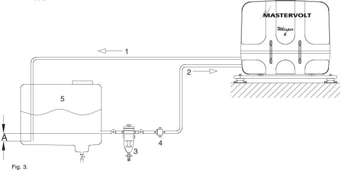
Both supply and return fuel pipe lines should be appropriate material and 8 mm outer diameter tubing. The quality of the tubing of fuel pipes could be submitted to local regulations depending on the application of the vessel.
