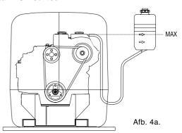
The tank has to be placed close to the generator. When it is mounted above the top of the manifold the liquid in the tank will be drained when the cap on the manifold is taken off.
